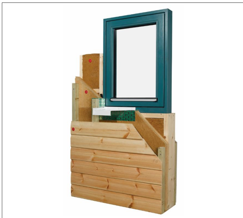
Figure 1 Isorooft / Pavatherm-Plus Sheathing Boards within a system
